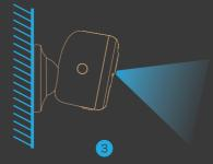
Attach the camera to the bracket and adjust the angle to cover the surveillance area. Do make sure the camera is within the Wi-Fi range.
