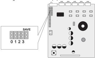
Setting method: short-circuit is "ON", open-circuit is "OFF"; add the four numbers of the four switches correspond, the result is the level No.. Set the numbers needed to the "ON" position. As below fig. Showing, it is the level 10..
