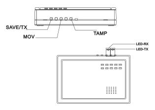
B. Keep pressing CLR-RX and MOV buttons on the transmitter need to set as entry data base, and then press TAMP button, LED-RF and LED-FS light up after alternate flashing, release CLR/RX and MOV buttons, LED-TX light, LED-RF, LED-FS alternate flashing, transmitter enter entry data base mode, in order to avoid false operation, before LED-RF and LED-FS light simultaneity, release any one of CLR/RX or MOV will cancel operation.
