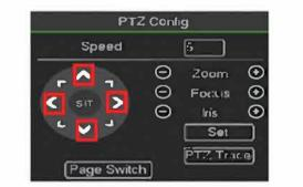
Step 8: Click - + - - + to change the focal length of the motorized lens.
