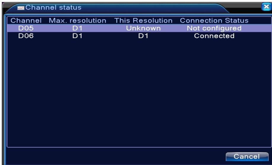
Channel status interface under full digital mode (One of the channel without device)
