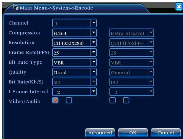
Picture 4.16 Encode setup
