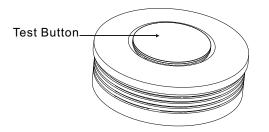
The D-SMOKE detects smoke and wirelessly transmits a signal to a receiver (control panel). It also has a built in buzzer to warn people in the immediate vicinity and the function of voice prompt. For testing purposes, the detector is equipped with a testing button. The detector makes regular autotesting and reports its condition to the system regularly for full supervision.
