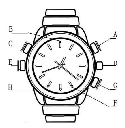
A,On/Off B,Indicator C,Mode D,Time Reset E,USB Interface F,IR Sensor G,Mic H,Lens
