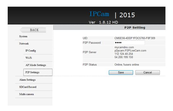
Here the P2P configuration can check Device UID and Password(Default 88888), and change the camera password.
