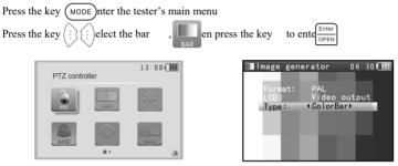
In the "color bar generator" mode, both PAL / NTSC format's color bars image can be output by the tester's "Video OUT "and received by the tester's "Video IN" port to display the video input and output .
