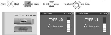
Turn on the blue cable tracer, use its copper pointer to touch all the cables in the bundle. User is searching at the other end. The cable that gives off the loudest tone is the cable connected to the tester. . Four Audio types can choose. The blue cable tracer has LED lamp. This is convenient for working in
