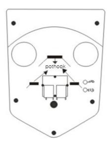
**7.3** On the back of the solar siren, there is some hanging buckle. Align the hanging buckle to the hanging hook on the plat to complete installation.
